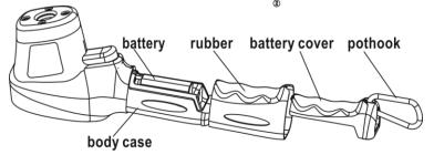
4.Replae the battery and put the rubber sleeve and the cover back.
