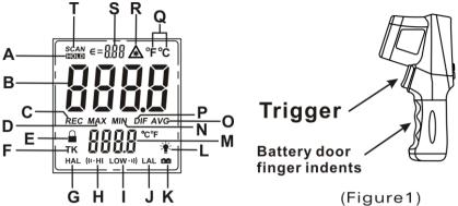
1. Remove the silica gel set, remove the battery cover screw with a screwdriver, and then slide out the battery door, install battery correctly. And Put back to the battery door screws and silica gel .Pull the trigger, LCD display reading & battery icon. Release the trigger and the reading will hold for 30 seconds.
